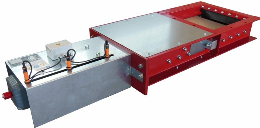
The **Flat slide gate TYPE SMFS GK Serie** will be mounted at the outlet of a silo or buffers to interrupt the free flow of bulk products. It ensures the best tightness of storing of grainy bulk products with a grain size up to 50 mm.
